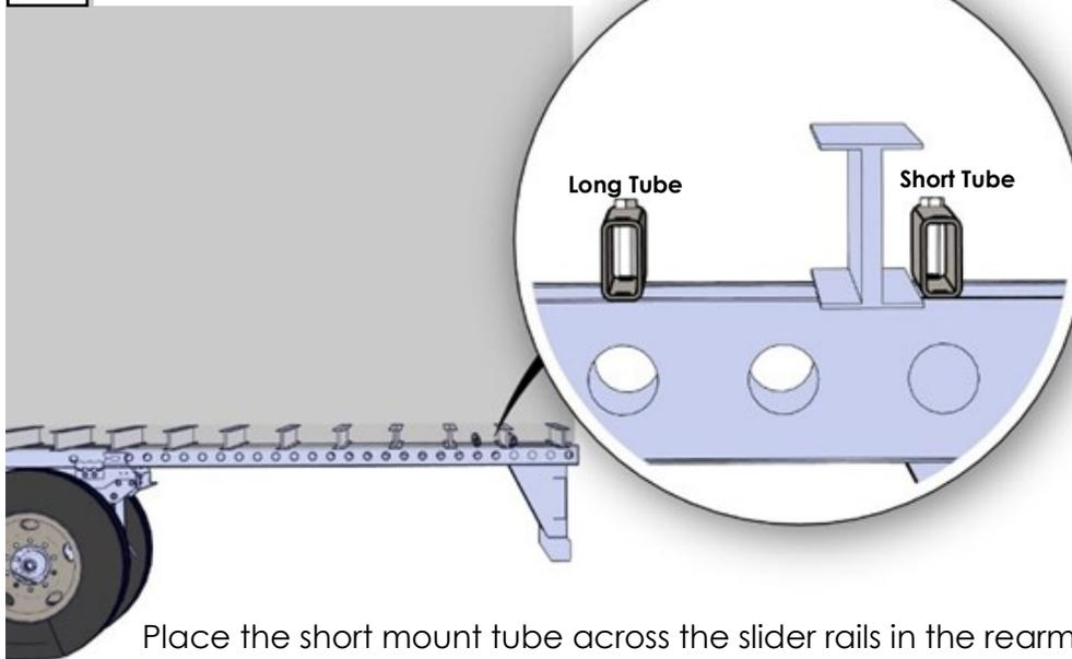
If you are unable to install the mount tubes in the rearmost position, move both tubes forward by one space.
